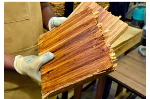
STEP 4 Compression into 8x8-inch tiles
