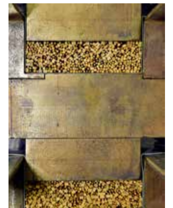
STEP 3 Baking under high heat for sanitisation and further removal of food debris
