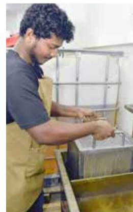
STEP 2 Soaking in an eco-friendly resin binder
