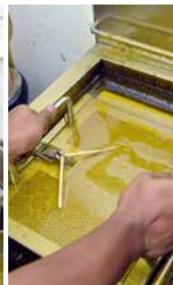
STEP 2 Soaking in an eco-friendly resin binder
